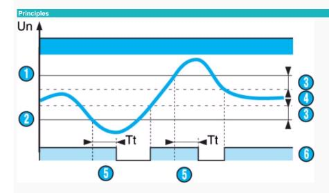
MUSF relays operate in window mode: they check that the controlled voltage stays between a minimum and maximum threshold.
